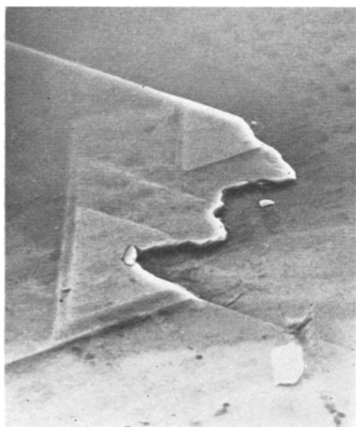
Figure 10 Triangular growth layers on (111) face of lithium ferrite.
