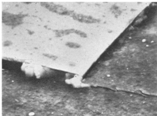
Figure 9 Growth step on magnetoplumbite crystal.
